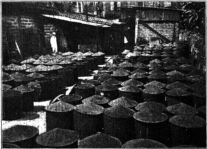
Fig. 2. The manufacture of toyo sauce. Soja beans fermenting in earthenware jars.
