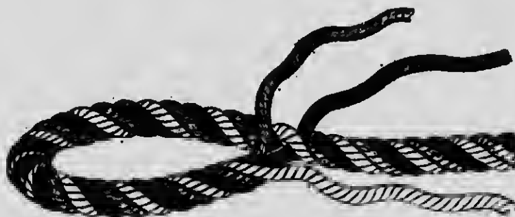
FIG. 18.—EYE-SPlice: FIRST STAGE.
