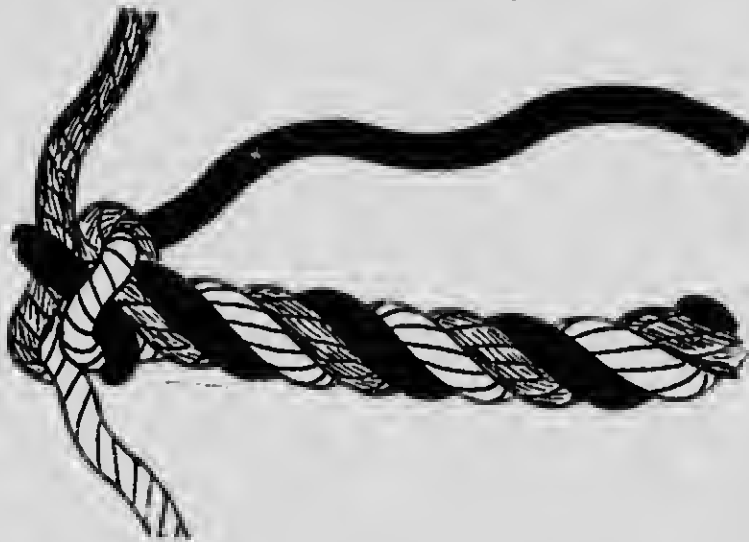
FIG. 30.—WALL AND CROWN : SECOND STAGE.
