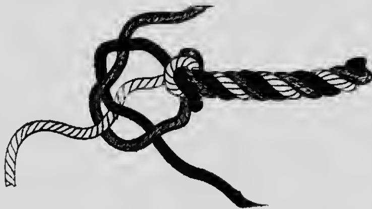
FIG. 29.—WALL AND CROWN: FIRST STAGE.
